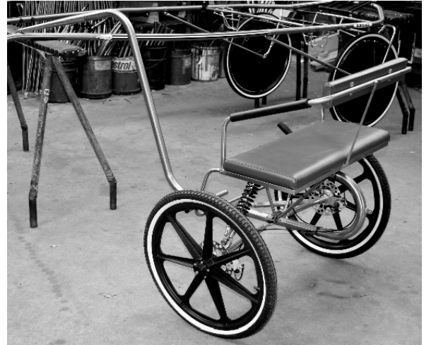
Photo above: Bench seat version of the mini dorsal hitch sulkie. [NB it is sitting at 90° to a racing sulkie so don't mix up the poles/shafts.]
